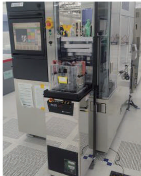
DISCO DFD6363 PLUS 500SDH(Heavy LiftArm)
